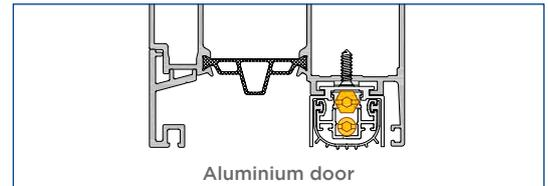
• **FEATURES** Mechanism (PATENTED) with the parallel descent of the moving profile with gasket, characterised by the DUAL ADJUSTMENT (screw E: descent - screw R: incline) for a strong even pressure on the entire length.
