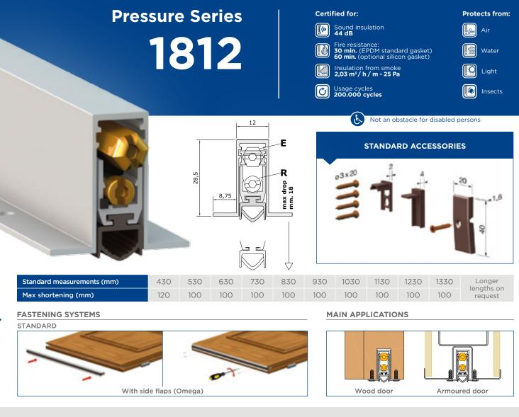
• **FEATURES** Mechanism (PATENTED) with the parallel descent of the moving profile with gasket, characterised by the DUAL ADJUSTMENT (screw E: descent - screw R: incline) for a strong even pressure on the entire length.
